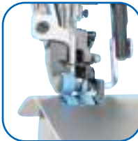
Alternating vertical movement mechanism
