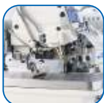
Presser foot arm with an open/close sensor
